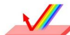
A red object reflects red and absorbs others colors of white light
