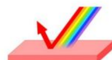
A red object reflects red and absorbs others colors of white light
